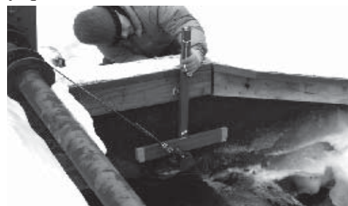
Amy Peterson measures the "before" gate height the traditional way, using Bruce's T-bar resting on top of the lifting point and read across the top of the bulkhead. This is the measurement recorded on the GLA website's Water Level report.
